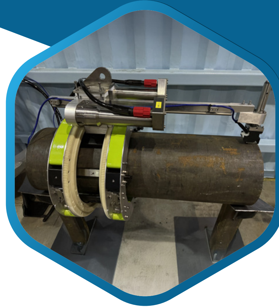
Automated Ultrasonic Testing (AUT)
