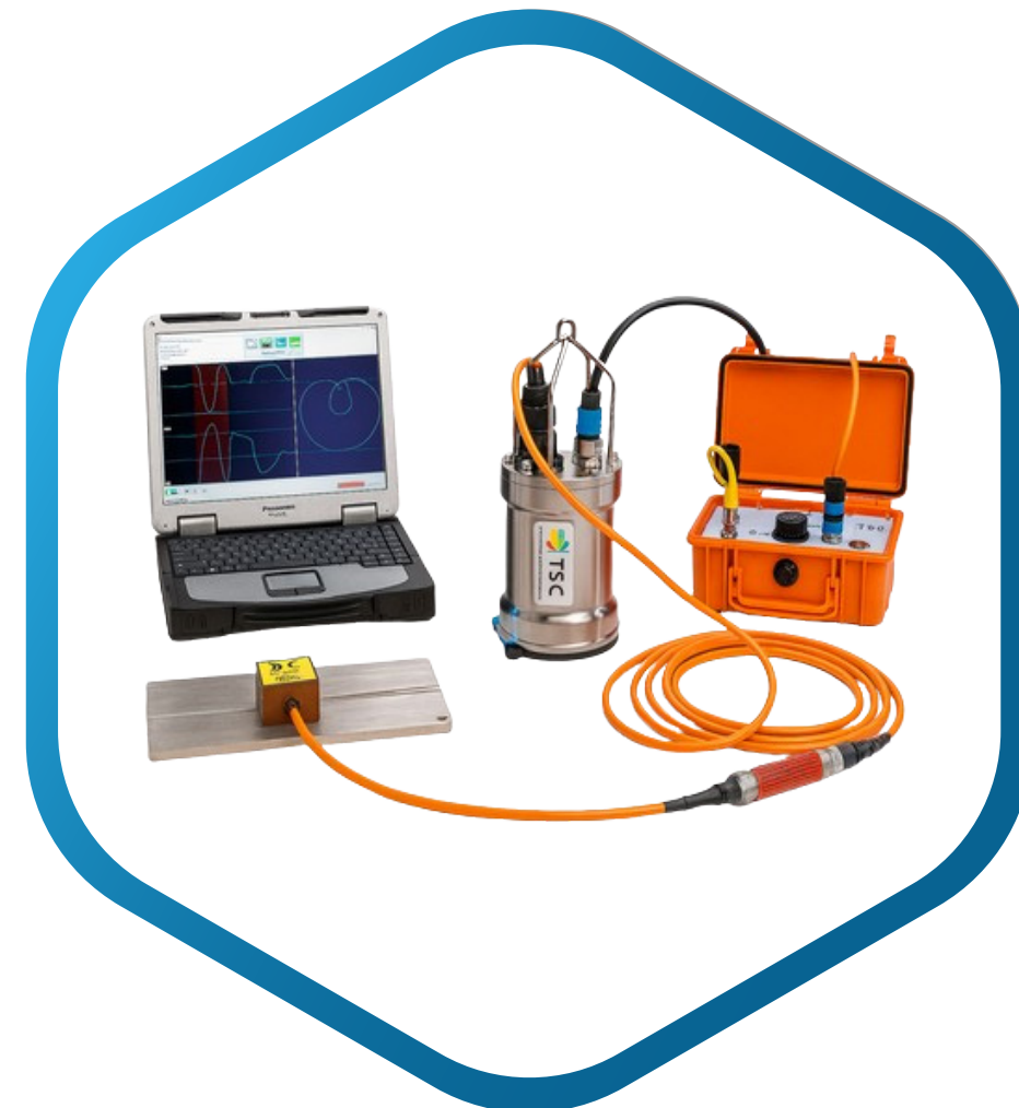
U31D Subsea ACFM® Inspection Technology
